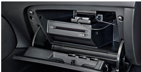
Mobile Phone Charging Station with Antenna Coupling
