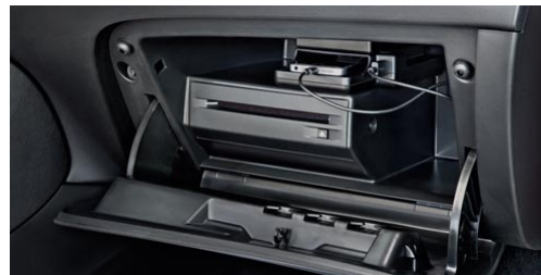
Mobile Phone Charging Station with Antenna Coupling
